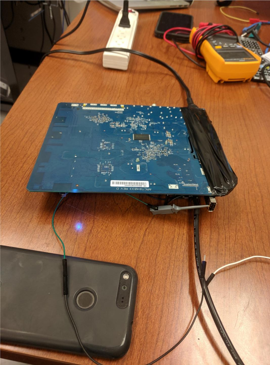
The green-black jumper cable is soldered to Ground on one side, and the other end is left floating. It will be used to poke at the memory chip.
