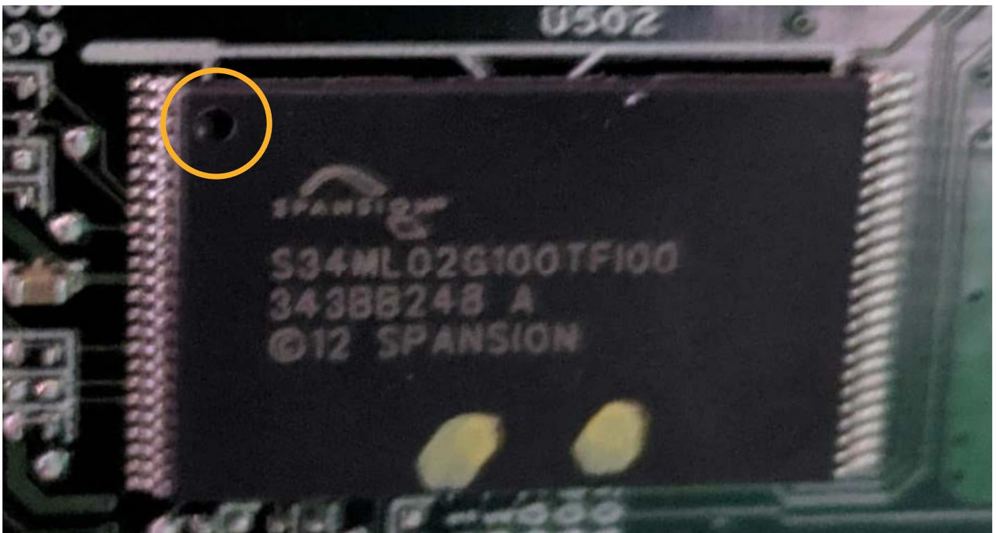
A description of the pins can be found in the relevant datasheet of the chip (Google the label written on the chip to find it). The pinouts are usually fairly standard; a typical one would look something like the one below. It is also good to know that pin number 1 is identified by a marking on the chip (a recessed circle, highlighted in orange in the top left corner in the picture on page 2).
