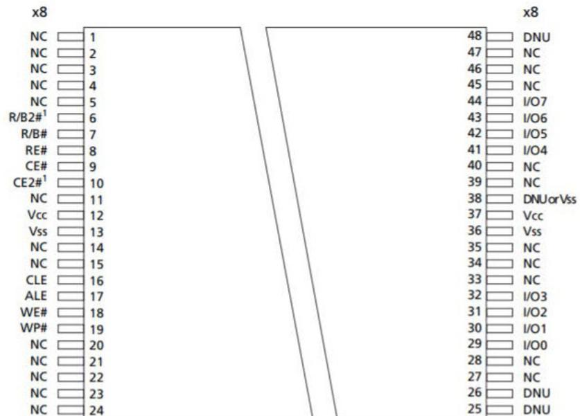
Notes: 1. CE2# and R/RB2# are available on 8Gb 2-CE# devices and 16Gb devices only. These pins are NC for other configurations.
