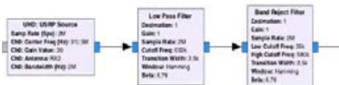
Figure 3: Band filtering to obtain narrow RX window
